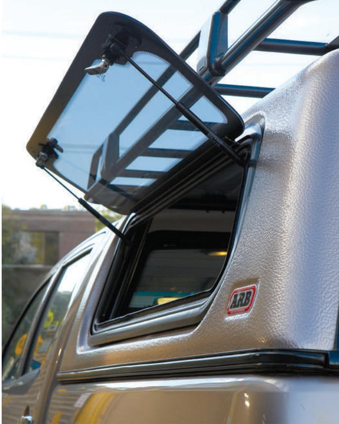
Lift up side windows allow easy access from the side of your utility. This option is available on one or both sides of the vehicle. All lift up windows are externally lockable with keyed alike access to the rear door.
