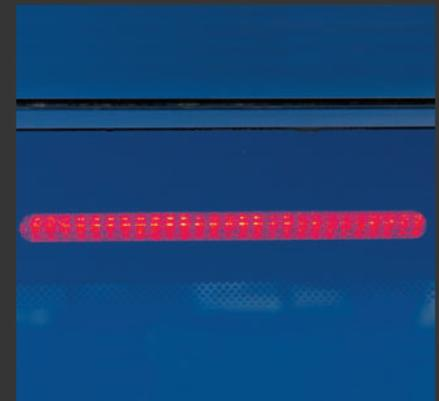
An LED brake light is fitted to all our Navara canopies, providing high output with low current draw.
