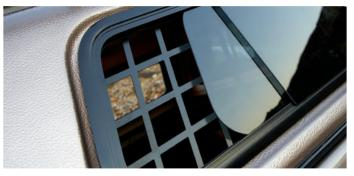
Laser cut from solid steel sheet and powder coated, security mesh is available for all sliding windows for extra security. It is also available to go over the front window of the Navara to protect cab occupants from equipment stored in the canopy.
