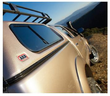
Sliding side windows are manufactured with tempered and tinted safety glass. Flyscreens can be fitted to these for increased practicality, especially if the vehicle is to be used as an occasional sleeping area.
