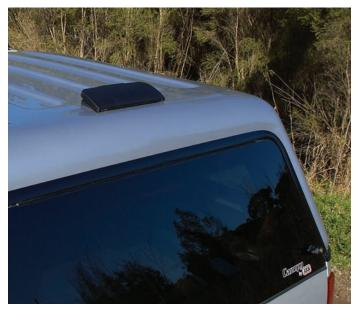
The innovative slimline, high flow canopy vent is the ideal solution to reduce dust ingress and improve airflow for your Classic canopy. With the vent facing the front of the vehicle, the canopy interior is pressurised, reducing dust from entering the area via the rear door or tailgate when travelling off road.
