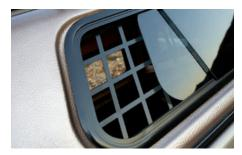
Laser cut from solid steel sheet and powder coated, security mesh is available for all sliding windows for extra security. It is also available to go over the front sliding window to protect cab occupants from equipment stored in the canopy.
