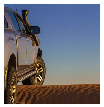
ARB protection steps offer similar benefits to conventional side steps, such as improved vehicle access and a reduction in stone chips caused by road debris. Unlike most other brands of steps, they act as a strong barrier between your vehicle and rock ledges encountered in off road driving, and are far less likely to sustain damage. Protection steps without the front side rail are also available as an alternative option for your Mazda BT-50.
