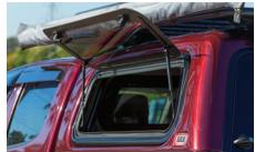
Lift up side windows allow easy access from the side of your utility. This option is available on one or both sides of the vehicle. All lift up windows are externally lockable with keyed alike access to the rear door.
