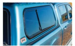
Sliding side windows are manufactured with tempered and tinted safety glass. Flyscreens can be fitted to these for increased practicality, especially if the vehicle is to be used as an occasional sleeping area.
