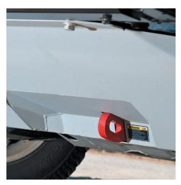
ARB's vehicle specific recovery point range offers a safe and secure winching point during vehicle recovery. Manufactured from steel plate, the recovery points are designed to take the guesswork out of shackle and snatch strap selection, with all ARB recovery points specifically rated for use with a 4.75t bow shackle and 8,000kg snatch strap.
